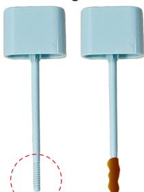
Ensure the probe tip is lightly coated with the sample.
