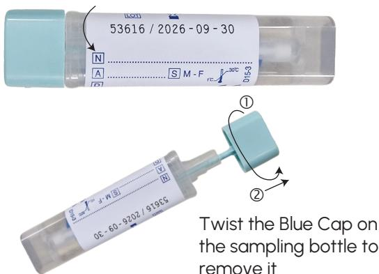
Twist the Blue Cap on the sampling bottle to remove it
